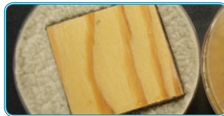
Wood sample piece with coated BactiBlock® R1.47: Efficient coating against Aspergillus Niger
