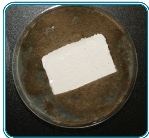
Silicone sample piece with 3% BactiBlock® 101 R1.47: We observe the high effectiveness of the additive against mold.
