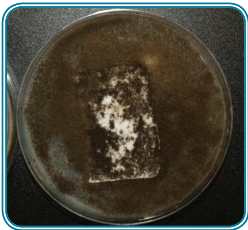
Control silicone sample piece without BactiBlock®: We observe the fast growth of Aspergillus niger after 4 weeks
